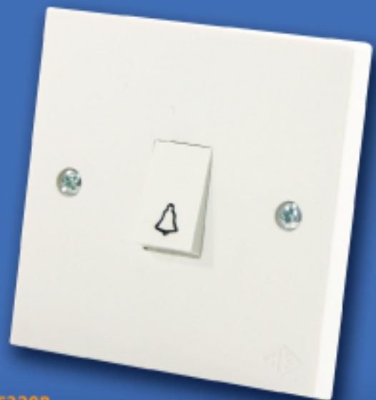
F230B 10 Amp. Push button Retractive switches. Bs. 3676 1 Gang marked with bell symbol can be wired for (N/O) or (N/C)
