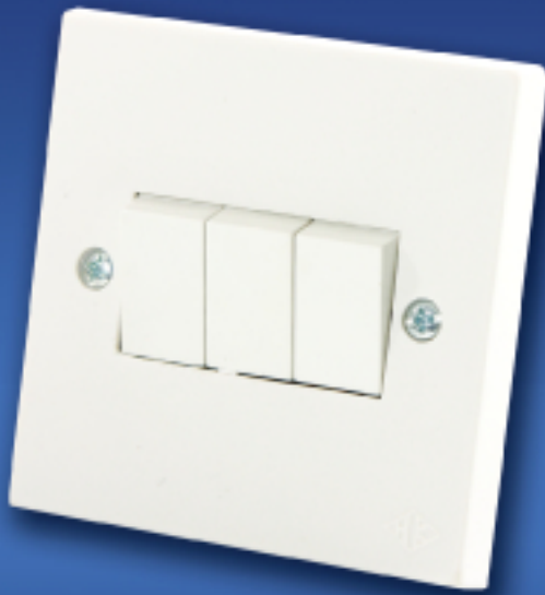
F242/1 , F242/2 10 Amp. Flush mounting type. Bs. 3676 3 Gang 1 Way 3 Gang 2 Way both suitable for fluorescent fittings
