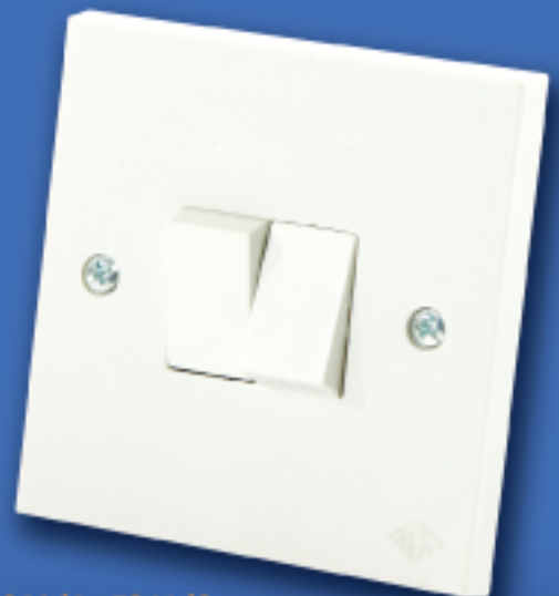
F241/1 , F241/2 10 Amp. Flush mounting type. Bs. 3676 2 Gang 1 Way 2 Gang 2 Way both suitable for fluorescent fittings
